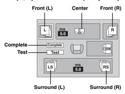
A Test signal is output from each speaker in a clockwise motion. Signals are also output from the front speakers, but they cannot be adjusted. Use this when adjusting other speakers for comparison. When the test signal is being output, press  $[\blacktriangle, \blacktriangledown]$  to lengthen the time of the test signal.
