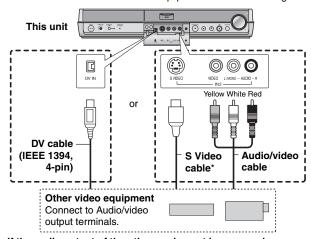
If the audio output of the other equipment is monaural Connect to L/MONO on the IN2 input terminals at the front.
